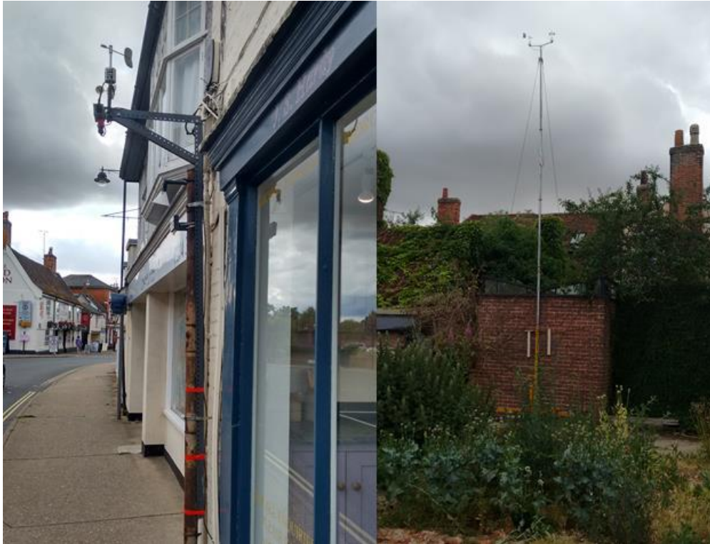
Figure 2: Wind speed and direction masts, Melton Hill (2 metre and 9 metre masts)
