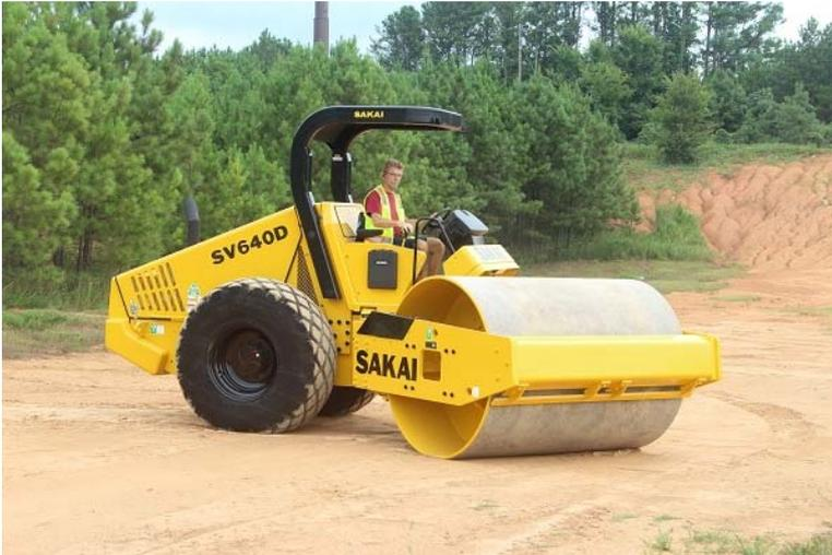
Material which has been compacted to a dry density less than required or at a moisture content outside the tolerable range shall be removed or reworked and re-compacted until the required properties are achieved.
