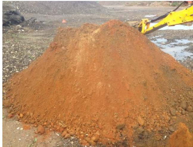
Photo 52: Arisings from trial pit TP10.
