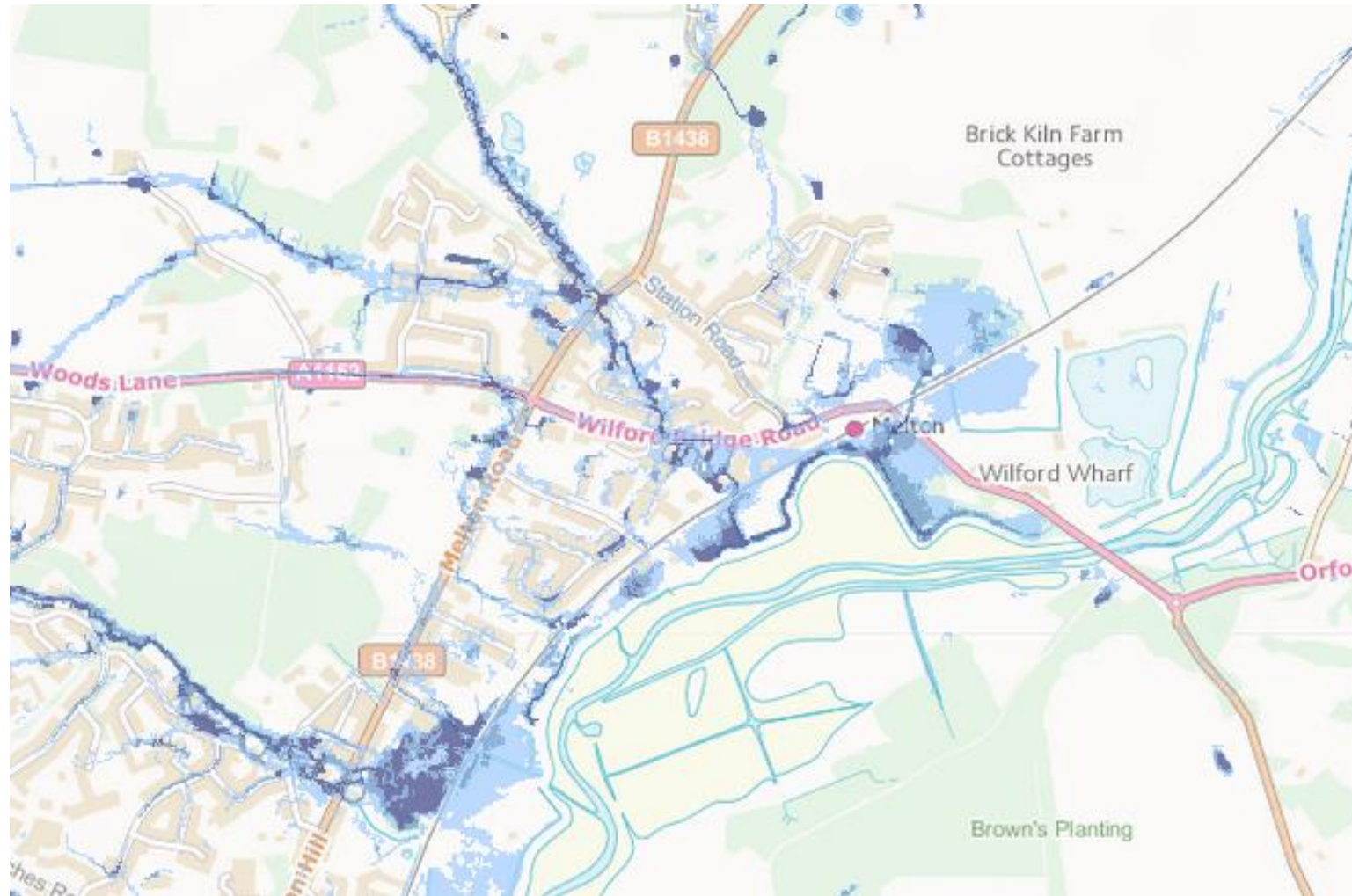
Figure 3.4: Risk of surface water flooding
