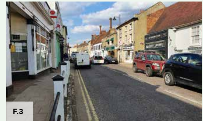
Figure 02: The northern point along the High Street creates pinch points due to the narrow carriageway, approximately 4.5m, affecting the sense of safety for pedestrians and cyclists.
