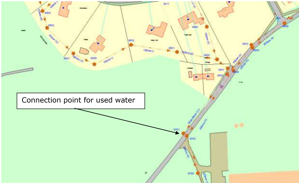
Figure 1: Showing your used water point of connection at manhole 9701 with a Cover Level of 12.018m, we do not have the Invert Level on record
