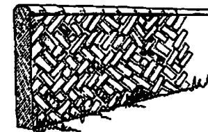
A random wall of brick and flint with a clay semi-circular coping.
