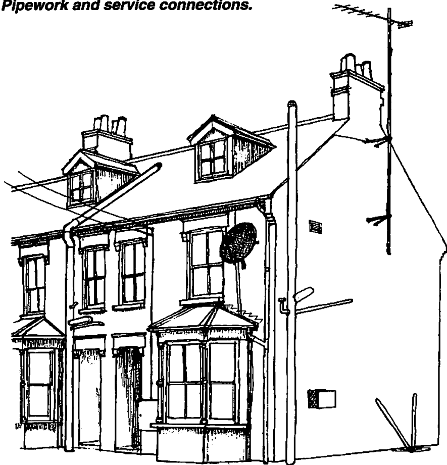
External pipework, meter boxes and various other additions can disfigure otherwise attractive old buildings.
