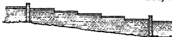
Stepping a wall down a slope has a jagged appearance and should be avoided.
