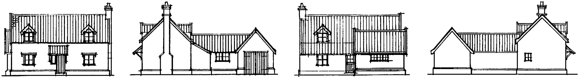
1. A 1½ storey cottage with a typical vernacular form, incorporating a rear lean-to (or "outshot") and single storey range linked to a garage.
