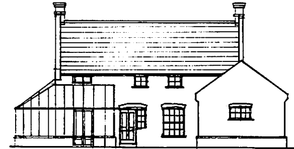
White painted timber windows, joinery and conservatory.
