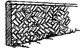
A random wall of brick and flint with a clay semi-circular coping.
