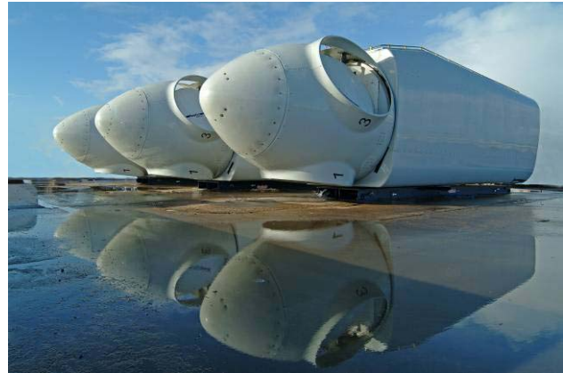
Figure 4-2: Nacelles on the Quay-Side
