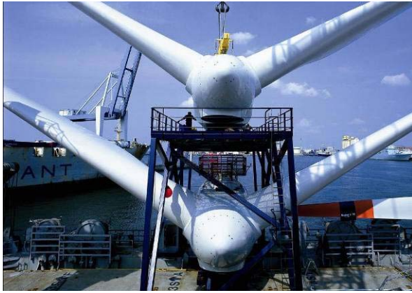
Figure 4-1: Stacked Nacelles with Blades
