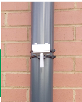
ESC OPCube continuous air quality sensor measuring \text{NO}_2 , \text{PM}_{10} and \text{PM}_{2.5}
