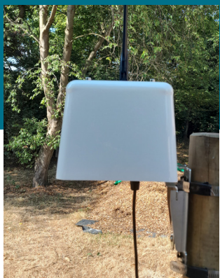
ESC OPCube continuous air quality sensor measuring \text{NO}_2 , \text{PM}_{10} and \text{PM}_{2.5}
