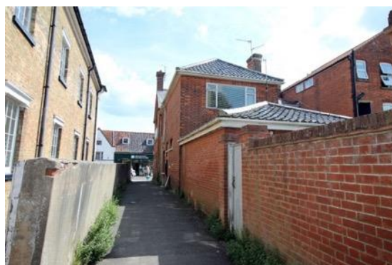
Woodleys Yard: This simple service lane has lost texture and visual interest with the use of modern cement render on an earlier brick wall. There is some evidence of damage to the brick as a result of water ingress.
