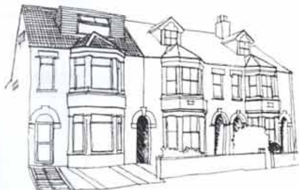
Loss of original details, including the addition of an overlarge dormer has seriously damaged the appearance of the house on the left.
