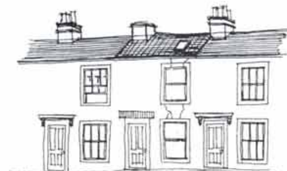
Unsympathetic alterations to roof and chimney.
