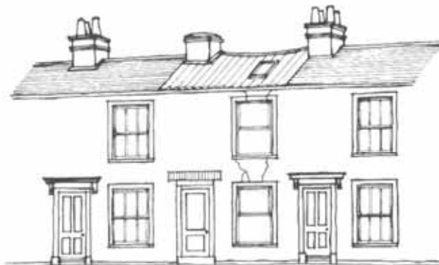
Ill considered modernisation, including re-roofing with heavy concrete tiles, can have disastrous effects both visually and structurally.
