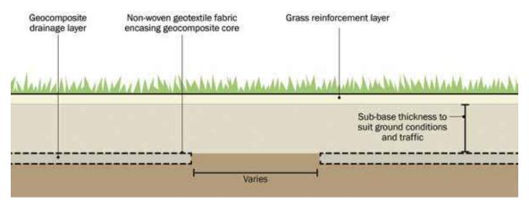
Figure 30.5 Geocomposite drainage strips used below permeable paving
