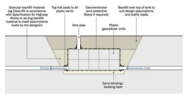
Figure 21.4 Schematic of 3D system in storage and attenuation mode
