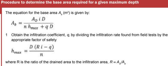
2 Find the porosity of granular fill material
