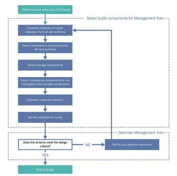
Figure 7.9 SuDS component selection process
