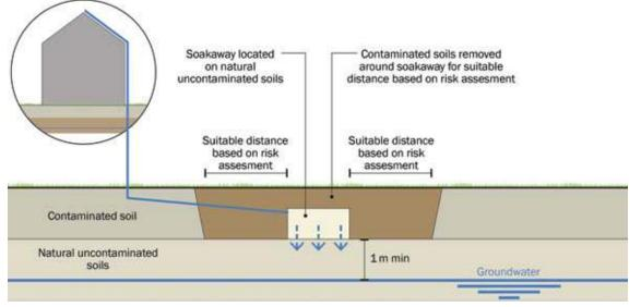
Figure 8.3 Locating infiltration systems beneath layers of contamination and/or removal of contaminated soils from around soakaways
