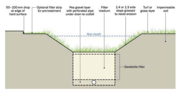
Figure 17.2 Typical dry swale
