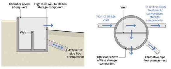
Figure 28.12 Conceptual design for engineered inlet flow divider
