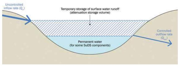
Figure 3.2 Controlling runoff rates using attenuation storage
