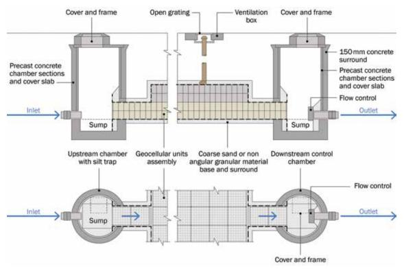
Figure 21.20 Example of sediment forebay
