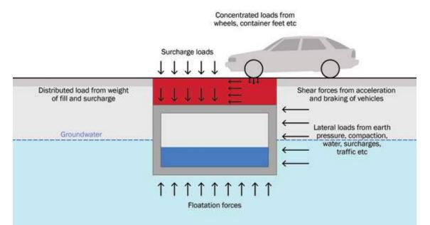
Typical loads that should be considered for any tank are shown in Figure 21.16.
