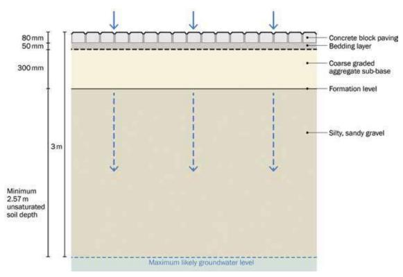
Figure C.7 Residential infiltration permeable block pavement
