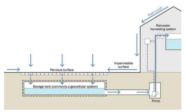
Figure 20.15 Example of rainwater harvesting system (from Interpave, 2010)
