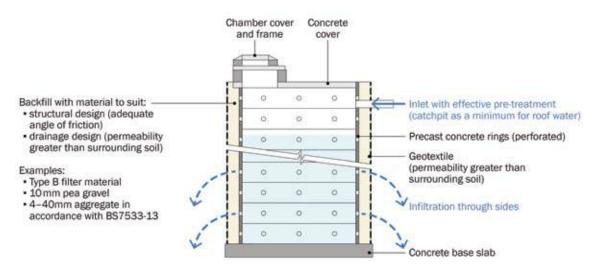
Figure 13.2 Soakaway details - concrete ring soakaway
