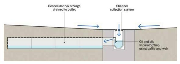
Figure 14.1 Schematic of a commonly used treatment channel
