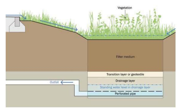
Figure 18.8 Anaerobic bioretention system
