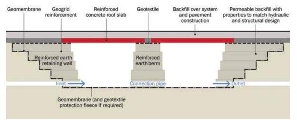
Figure 21.14 Typical layout of hybrid tank
