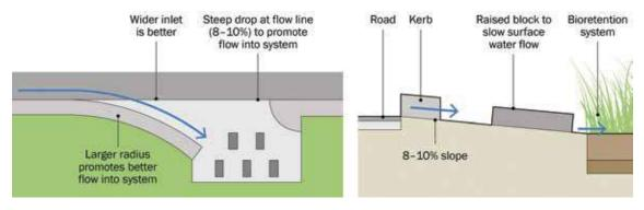
Figure 18.10 Inlets to a bioretention system as used in Lambeth, London (courtesy Lambeth Council)
