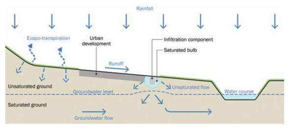
Figure 25.1 Typical surface water management infiltration system
