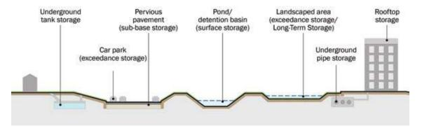
Figure 24.5 Examples of attenuation storage locations
