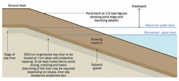
Figure 23.15 Details for a typical clay liner
