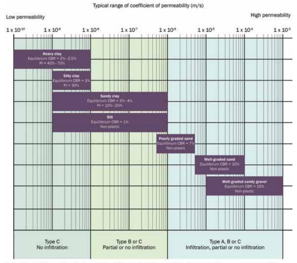
Note: A significant proportion of clay and silt (> 15% of particles less than 63 µm) will reduce the permeability and CBR values of sand and of gravels
