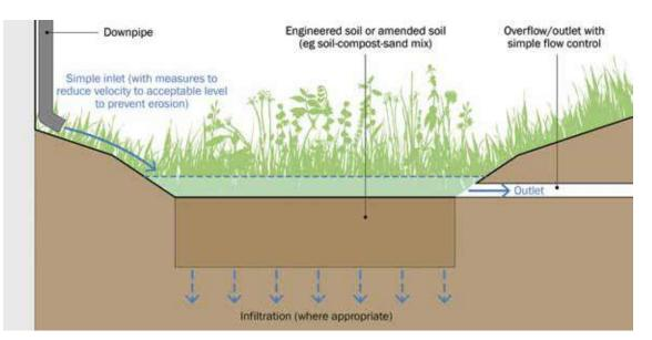
Figure 18.2 Section through a simple rain garden with outlet pipe
