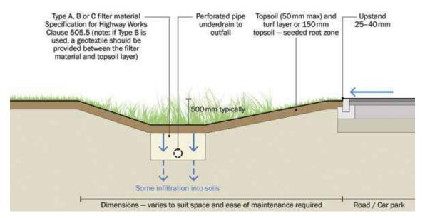
Figure 9.15 Swale detail
