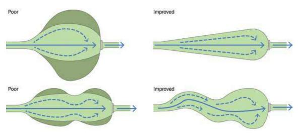
Figure 28.2 Examples of poor and improved inlet and outlet configurations
