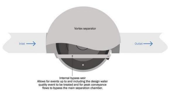
Figure 14.6 Hydrodynamic separator with an internal (or integral) bypass (courtesy Hydro International)
