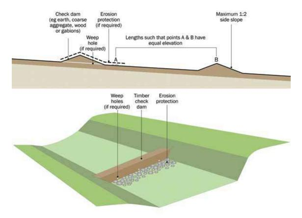
Figure 17.13 Typical check dam details
