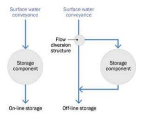
Figure 24.6 On-line vs off-line storage
