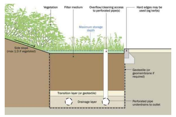
Figure 18.1 Components of a bioretention system
