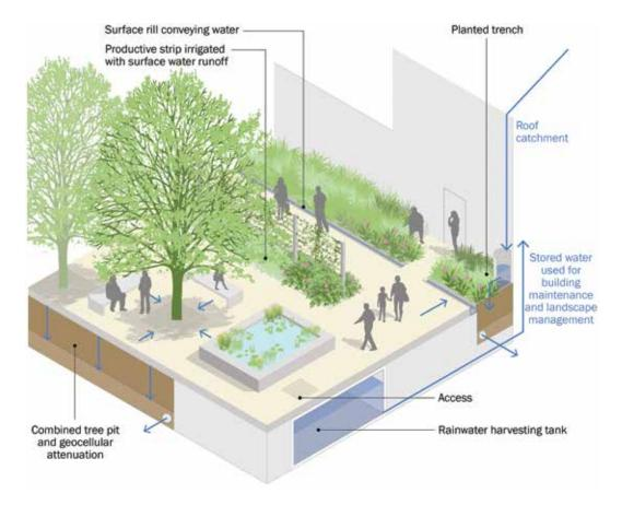
Figure 10.12 Communal space using runoff as a resource
