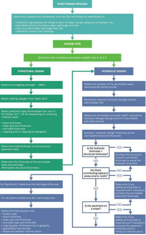
Figure 20.19 Pervious pavement design flow chart (after Interpave, 2010)
