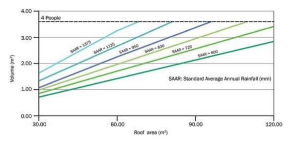
Figure 11.7 The simple method for sizing RWH tanks - for water conservation only (from BS 8515:2009+A1:2013)
