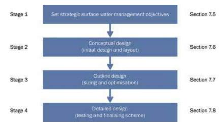
Figure 7.1 The four stages of SuDS design
