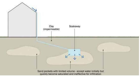
Figure 25.3 Local soil testing misrepresenting wider soil properties
