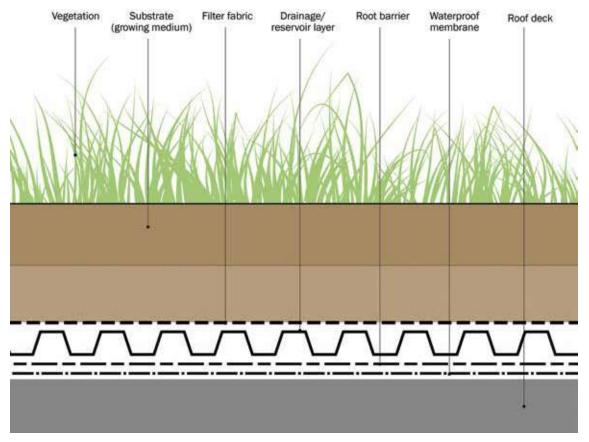
Figure 12.1 Section showing typical extensive green roof components
