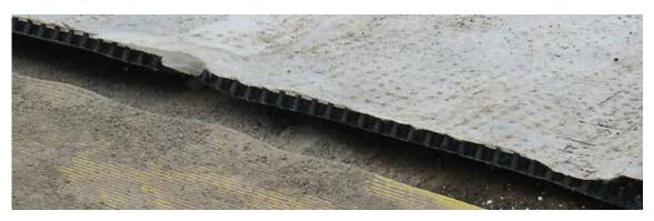
Figure 30.4 Geocomposite drainage layer (courtesy Stormwater Management Ltd and Geosynthetics Ltd)
