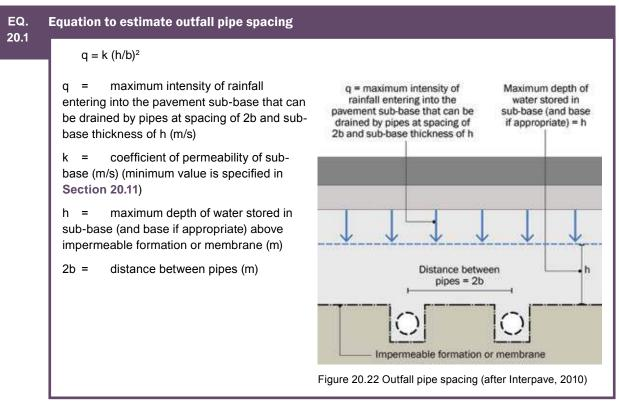
Water should flow horizontally through the sub-base to reach the outlet collection systems and there should be sufficient capacity in any aggregate to convey the rates of flow required. Horizontal water flows can very crudely be estimated using Darcy's law (ICPI, 2011) – **Equation 20.2**.
