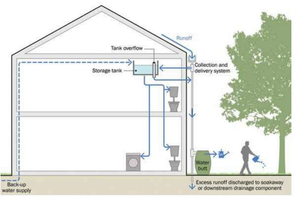
Figure 11.3 A conceptual gravity-fed RWH system
