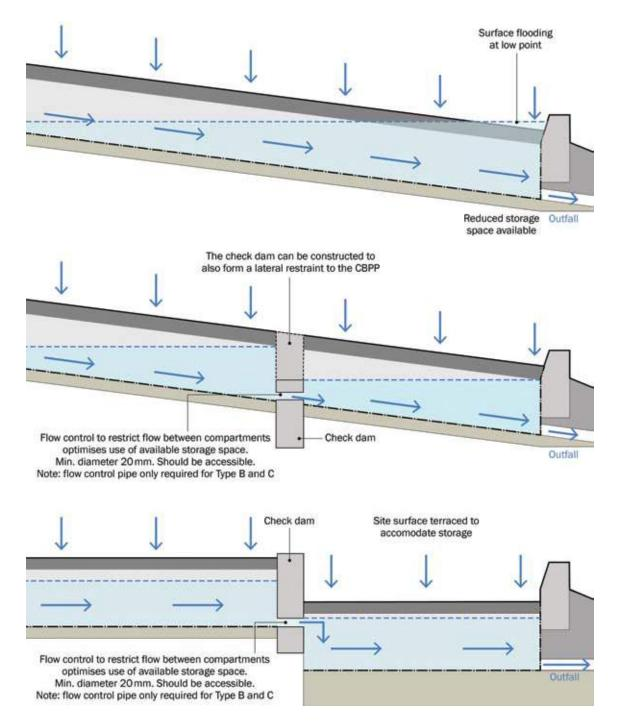
Figure 20.21 Control of water on sloping sites (from Interpave, 2013)
