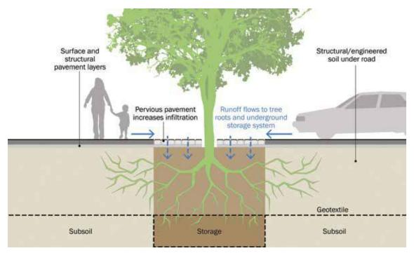
Figure 19.3 Collection of surface water runoff for trees
