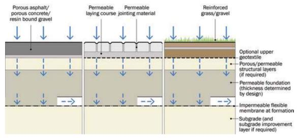
Figure 20.14 Pervious pavement system types: Type C - no infiltration
