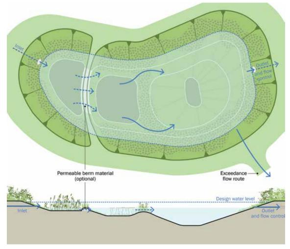
Figure 23.4 Plan view and profile of pond details
