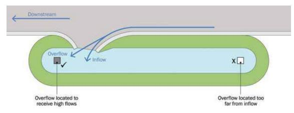
Figure 18.16 Inlet and overflow outlet configuration (small scale) (after Water by Design, 2012)
