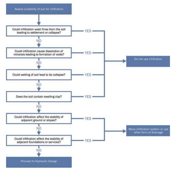
Figure 25.4 Decision guide for the use of infiltration systems
