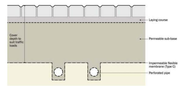
Figure 20.25 Perforated pipe outlets below sub-base
