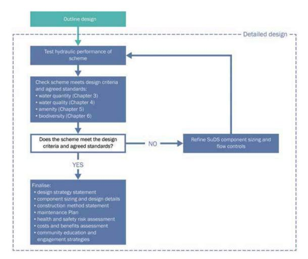
Figure 7.13 The detailed design process
