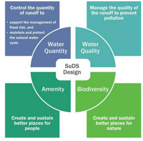
Figure 2.1 The four pillars of SuDS design
