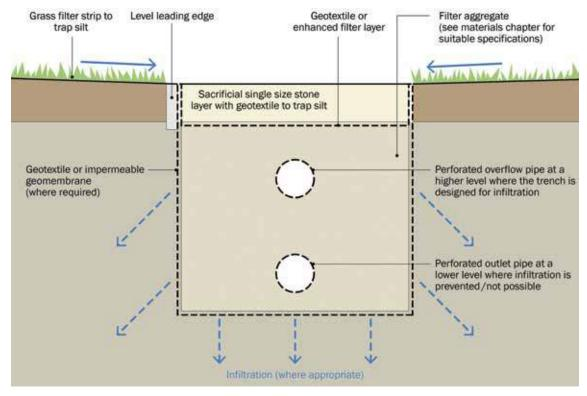
Figure 16.2 Filter drain schematic
