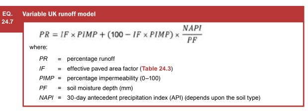
This equation effectively divides PR into the two contributions from paved and pervious surfaces. The impervious area runoff is obtained by using an "effective contributing area" proportion, IF (ie from surfaces that run directly into the drainage system). The original recommended values of IF are given in **Table 24.3**. However, IF values have tended to be applied at around 0.7 in practice in most models.
