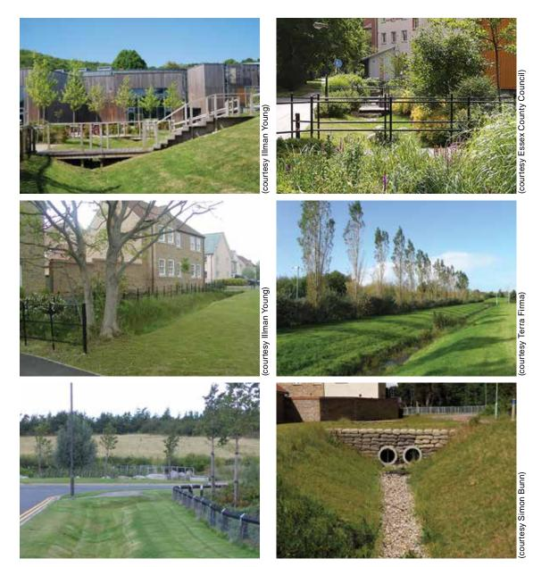
Figure 17.4 Examples of different swale types and designs
