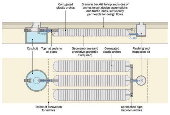
Figure 21.8 Typical layout of an arched system
