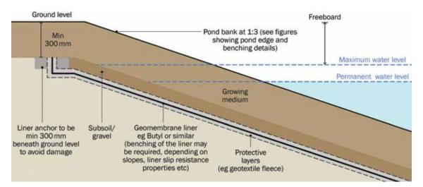
Figure 23.14 Details for a typical geomembrane liner
