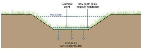
Figure 17.1 Typical conveyance/attenuation swale
