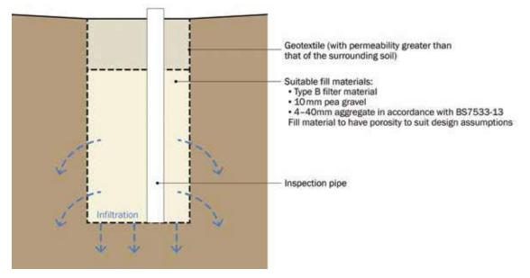
Figure 13.3 Infiltration trench
