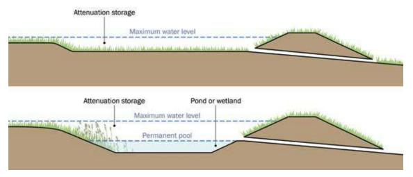
Figure 24.4 Attenuation storage in dry or wet components
