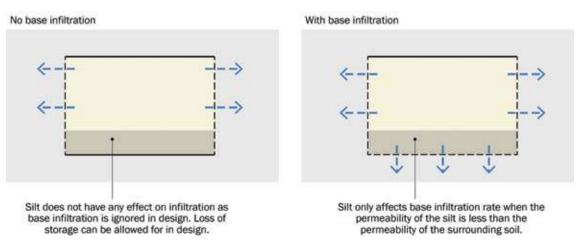
Figure 25.6 Effect of silt on performance of infiltration
