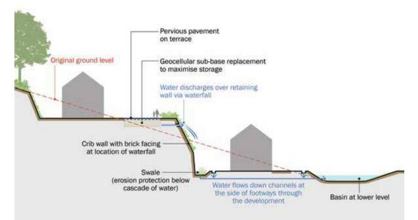
Figure 8.6 Cross-section showing example SuDS on a sloping site
