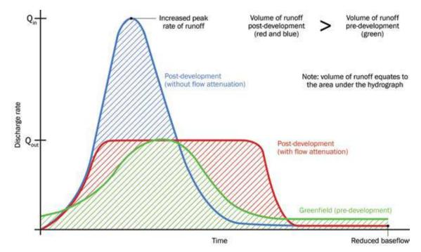
Figure 3.1 Example of a runoff hydrograph
