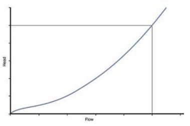
the chance of oils being transported Figure 28.13 Head–discharge relationship for a simple orifice plate (courtesy Hydro International)
