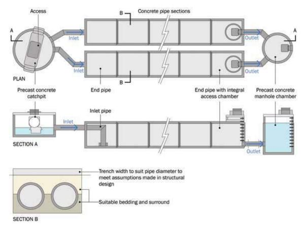
Figure 21.10 Typical layout of concrete pipe system
