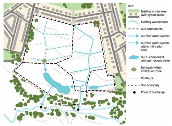
Figure 7.6 Defining surface water sub-catchments
