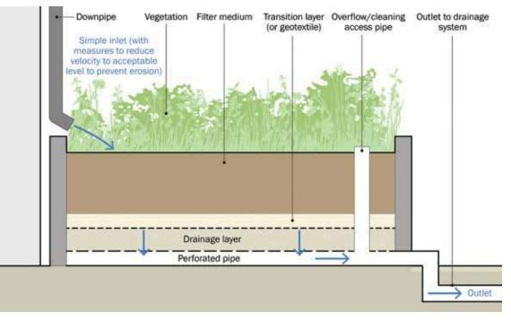
Figure 18.5 Section through a raised planter
