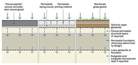
Figure 20.12 Pervious pavement system types: Type A – total infiltration
