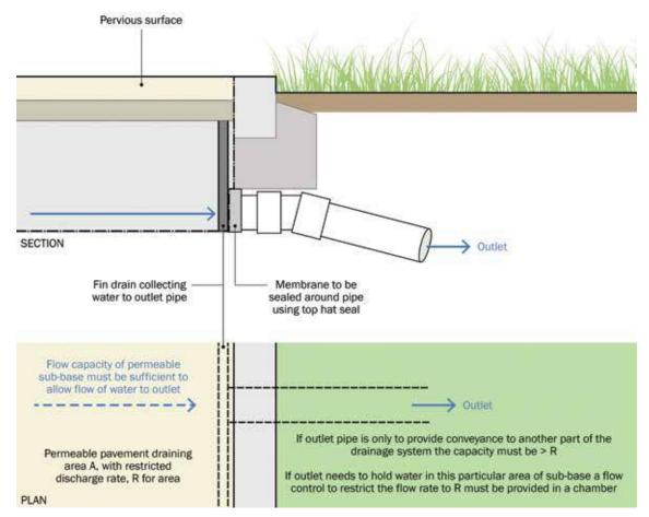
Figure 20.26 Fin drain outlet from pervious surface sub-base (from Interpave, 2010)
