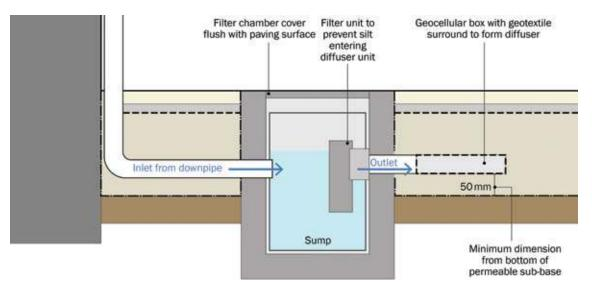
Figure 20.24 Flow diffuser to distribute roof runoff into permeable sub-base (from Interpave, 2013)
