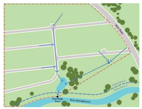
Figure C.3 Main flow routes and discharge points
