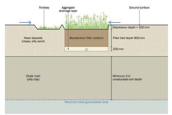
Figure C.9 Civic street infiltration bioretention systems
