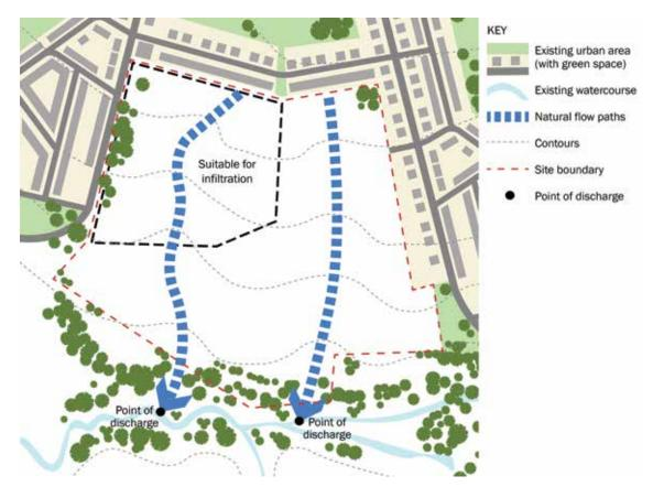
Figure 7.4 Characterising flow routes and discharge points
