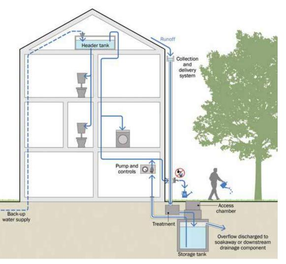
Figure 11.4 A conceptual pumped rainwater harvesting system
