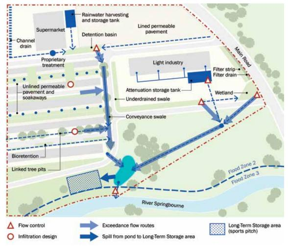
Figure C.5 Proposed flow controls and exceedance flow routes
