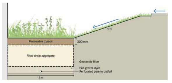
An underdrained swale (without lining) can be assumed to deliver Interception for 25x its area which is > 4.1 ha.
