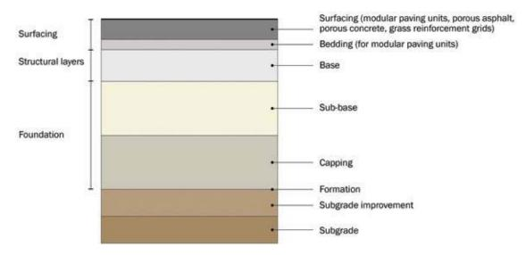
The main layers that are placed to form a road pavement are shown in Figure 20.23.
