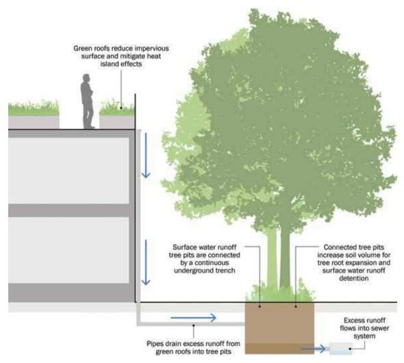
Figure 19.12 Integrated system of trees and green roofs
