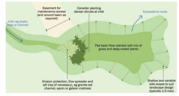
Figure 13.4 Plan view of infiltration basin
