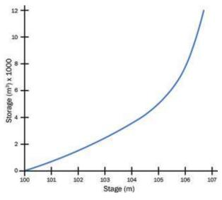
Figure 24.7 Example of a stage-storage curve
