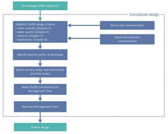
Figure 7.3 The conceptual design process
