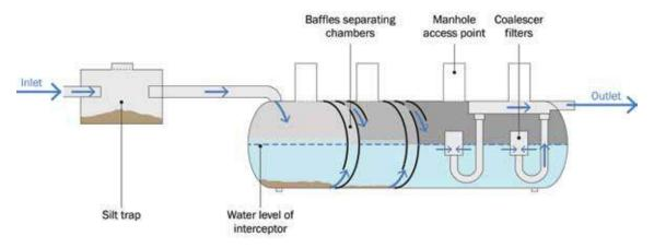
Figure 14.11 Outline diagram of a prefabricated, multi-chamber, full retention, Class 1 separator
