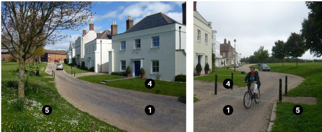
Figure 43 Examples of edge lanes in Dorchester, with low-speed roads shared between motor vehicles and cyclists, and opportunities for on-street parking (note: some localities may prefer clearly defined footways and parking bays).
