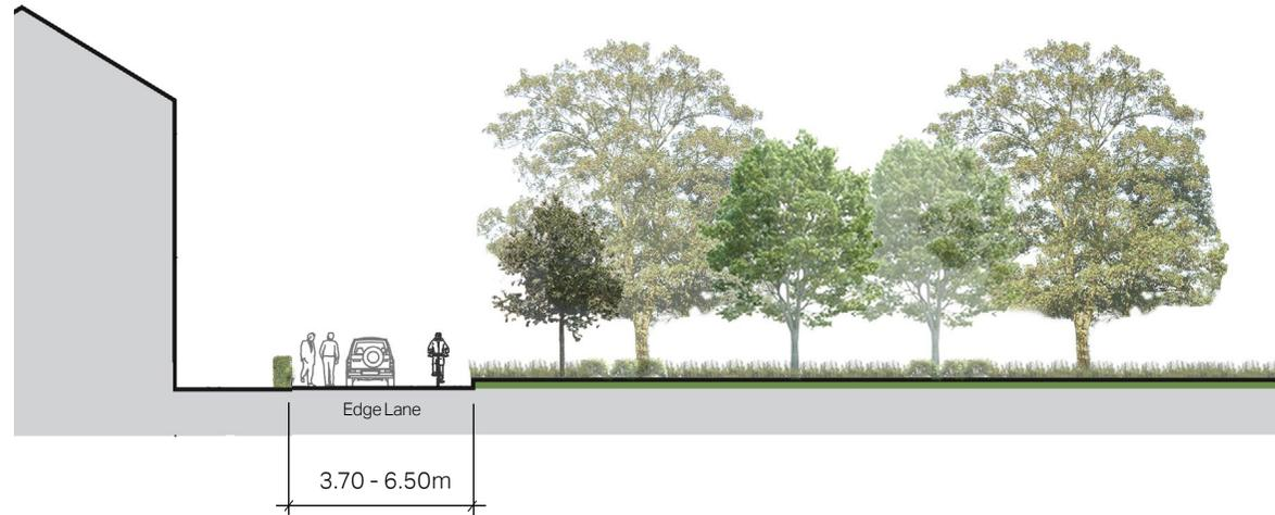
**Figure 36:** Cross-section to illustrate some guidelines for edge lanes.
