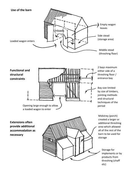
Figure 2 Diagram showing typical structure and use of traditional barn
