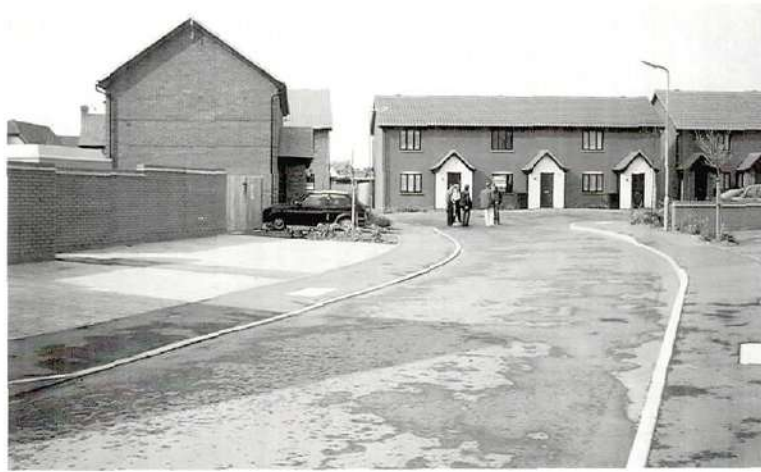
Unacceptable - unscreened and poorly detailed parking areas creating a very poor environment
