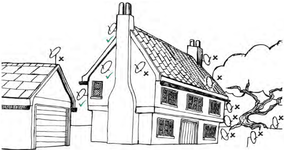
Diagram 2: Correct positioning of satellite dishes.
