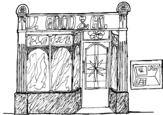
Diagram 5: Correctly located ATM.
